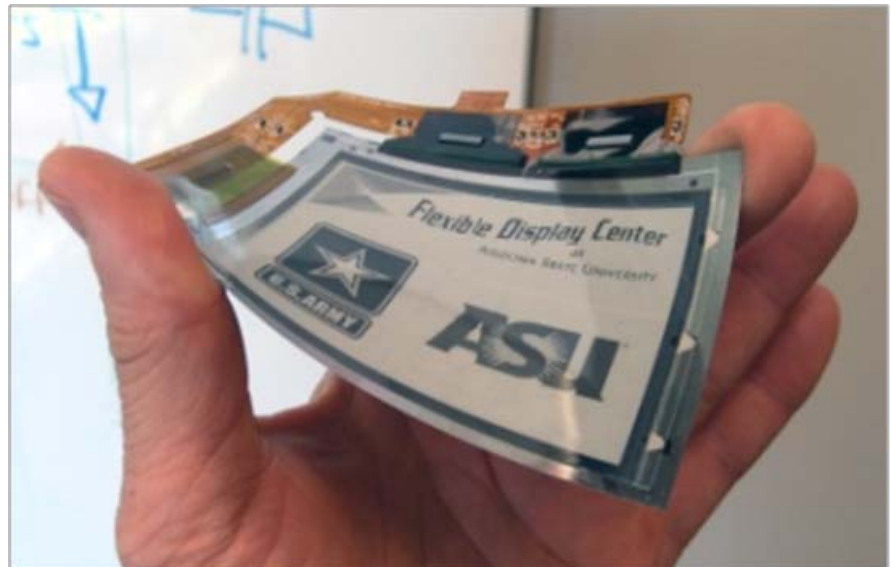
Figure 2: 3.8-inch QVGA E Ink display on Teonex Q65FA (Image courtesy of Flexible Display Center at ASU)
