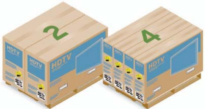
Using conventional cushioning foam (left), a large flat-screen television can be packed with only two units to a standard pallet. ARCEL resin (right) allows for cartons approximately half that size, easily doubling the yield.
