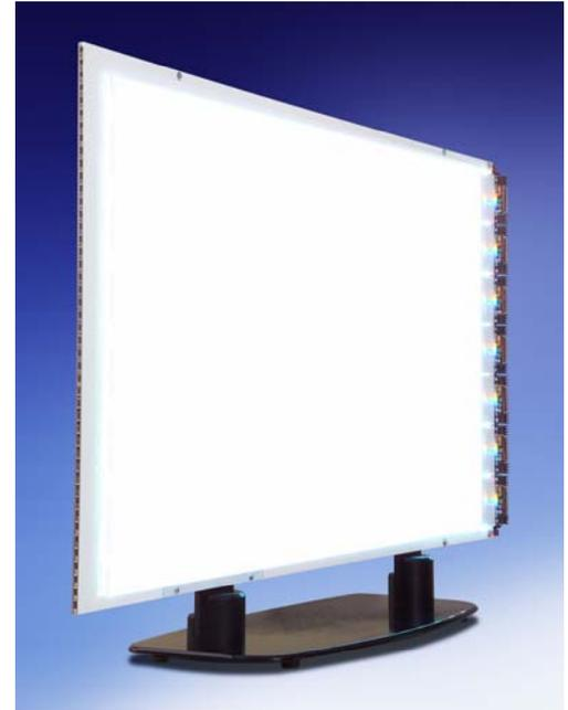
*The PhlatLight LED back light unit won the 2008 Display Component of the Year Gold Award from the Society of Information Display (SID). The PhlatLight 46-inch BLU is illuminated with eight light modules, each containing a single red, green and blue PhlatLight LED. The LEDs illuminate the BLU from the edges, not the back, enabling thinner designs.*
