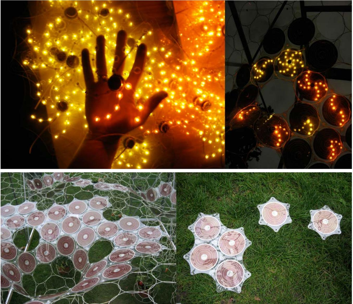
*A modular photovoltaic membrane was prototyped for the installation that can be clad to synthetic textile architecture to provide both shelter and shade from the sun during the day and once evening falls light is cast into the darkness using low-power micro LEDs with printed circuitry. Loop.pH will be developing this over the next 12 months as a low cost, high volume source of light for emergency shelter relief – in places where light and electricity are not provided.*
